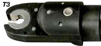
The 48ET tube nut wrench alternates the direction of rotation each time the lever is actuated. When rotating in reverse, the socket will stop at the open position.
